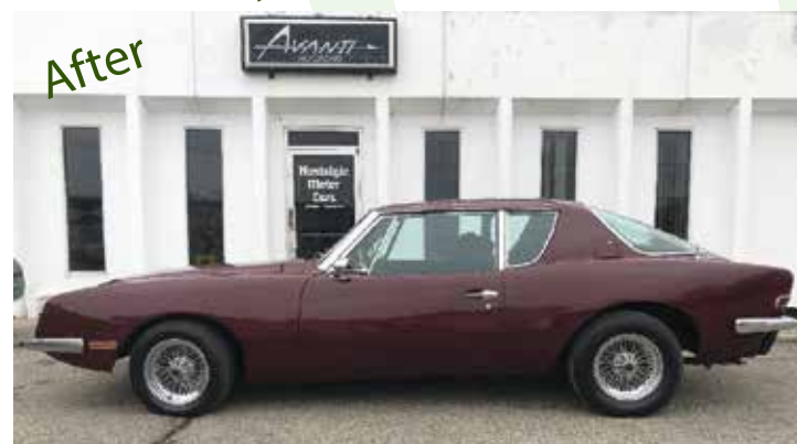
After: Front spring spacers removed, with 215-60x15 tires on the front and 245-60x15 tires on the rear.
