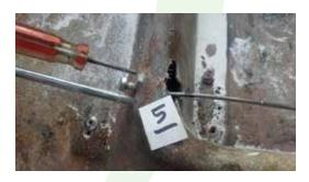
Grind the fiberglass floor area to be reglassed.
