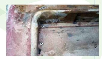
As I mentioned before, the original nut plate pop rivets were smaller and flat headed. They were also counter sunk to be flush with the surface. It would be very difficult to counter bore these holes to allow for a flush surface with the fiberglass and not necessary.
