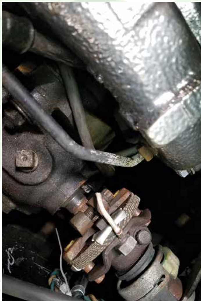
New Original Stock Rag Joint #1701886, Installed with jumper ground wire
