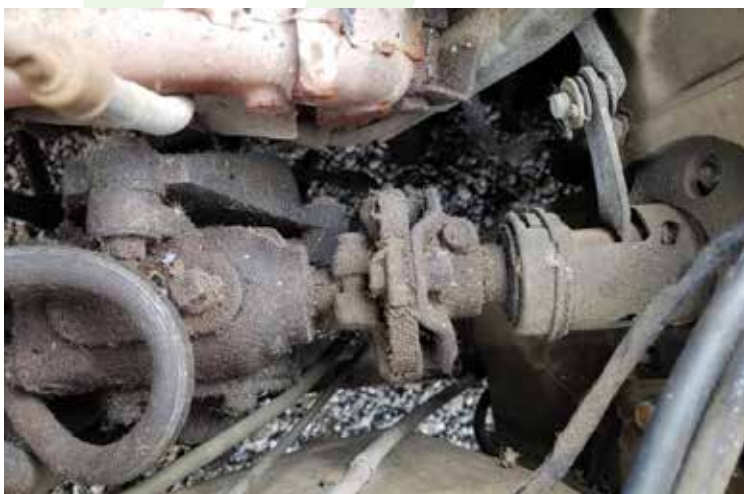
New Original Stock Rag Joint #1701886, Installed with jumper ground wire
