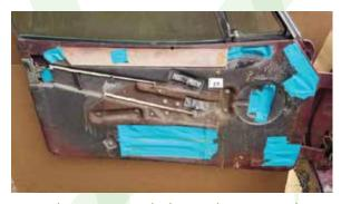
Tape up the remaining holes, and you're ready to reinstall the door panel.
