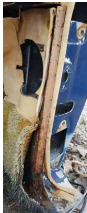
Photo of rusted kick pad retainer P#1347528x61
