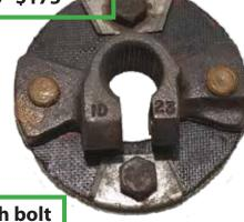
1700615 Special pinch bolt for 1701883 steering flange & insulator rag joint \$5
