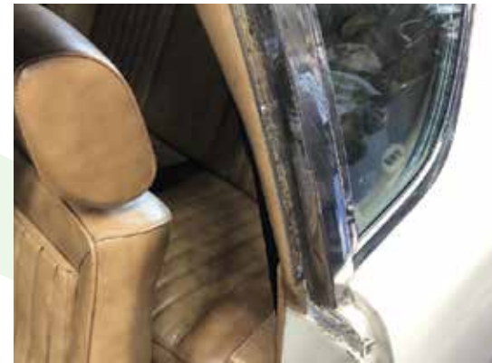
Stainless and Recess for Dog Leg Weather Seal
