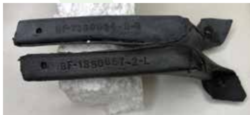
Studebaker designed the Dog leg molding, at left, Illustration # 2116-24 weather seal as a glued together, two piece seal, for good reasons.
