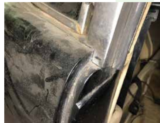
The dog leg weather seals illustration numbers 2116-24 and part numbers #1350856 and 1350857 were changed about half way through the 1983 Avanti model run.
