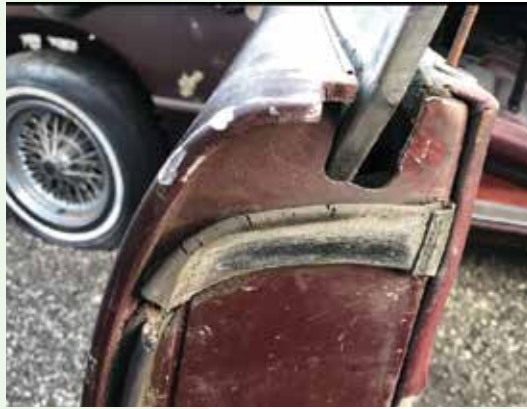
Above is a V-shaped upper dog leg weather seal.
