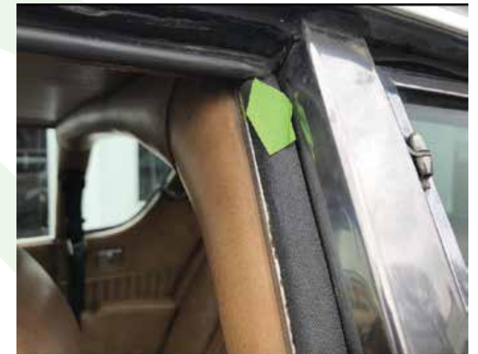
Upper Door Weather Seal Hole Location at the Top Back
