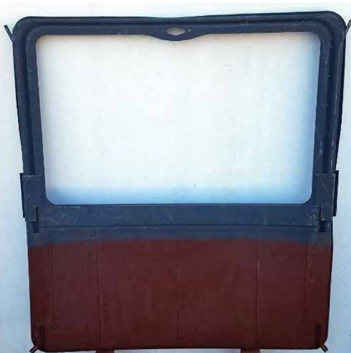
Please notice in this picture, the drain tube nipples, located at each corner
