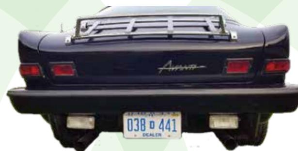
The 2nd style was needed as Avanti Motors took the back up lights out of the trunk lid and installed them on the rear fiberglass tail pan. The trunk lid now had amber turn signal lights where the back up lights used to be. Then they switched to red turn signal lights.
