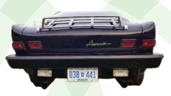
The 2nd style was needed as Avanti Motors took the back up lights out of the trunk lid and installed them on the rear fiberglass tail pan. The trunk lid now had amber turn signal lights where the back up lights used to be. Then they switched to red turn signal lights.
