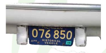
The 3rd style N.O.S. 1750989 still had the tab for Motors added a tab on each end of 1750760 to mount the back up lights, the back up lights were transferred and now were vertical on each end of the license plate bracket. This started sometime in 1984 through 1985.
