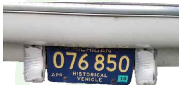
The 3rd style N.O.S. 1750989 still had the tab for the rear license plate light assembly, but Avanti Motors added a tab on each end of 1750760 to mount the back up lights, the back up lights were transferred and now were vertical on each end of the license plate bracket. This started sometime in 1984 through 1985.
