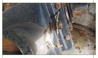
The heater assembly is now ready to remove. Rotate the assembly down and back away from the firewall. It will not come completely out as it will hit against the right lower dash support. Just simply take a large screw driver or small pry bar, insert it from the bottom up between the heater box and lower dash support. prying down so it will pass by the lower dash support.
