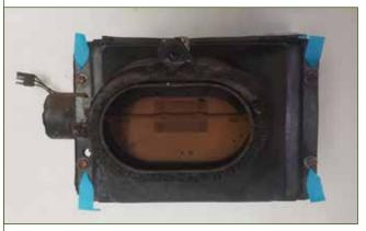
Remove the 4 bolts that hold the inner and outer housings together. Remove the old heater core. Wash the inside and outside of the housings.
