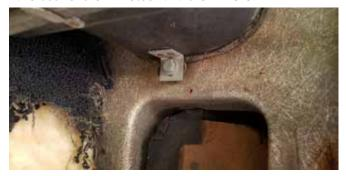
Remove the bolt from the right kick panel that holds the heater housing to the right kick panel. Note if this bolts spins, and won't come out, you will have to grind off the head to remove the heater assembly as it is threaded into a well nut part number WN-L6 which I have in stock if you need one.
