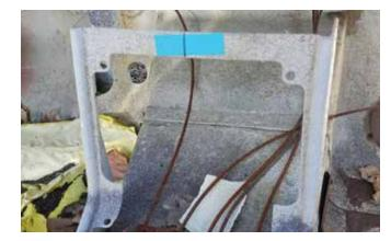
strip (about 1/2 wide) on the very top of the console directly below the dash. Remove the carpet from the console side Cut the very top of the console (it's about 1/2' wide) directly below the dash in the middle
