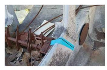
14. Draw a line on the console on a diagonal starting about 1" in front of the riveted bracket that holds the heater/fresh air cable assembly bracket to the console side and continue to the bottom console and angling forward.
