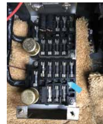
The blue arrows show 2 different spades that a wire can be plugged into for 12 volts, with the key in the on position. Note: check to make sure the spades on your Avanti only have 12 volts with the key on.
