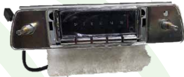
Radio with shafts adjusted to the N.O.S radio bezel.
