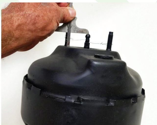
.985 off the flat face of the booster reach rod, to the tip of the adjustable end.
