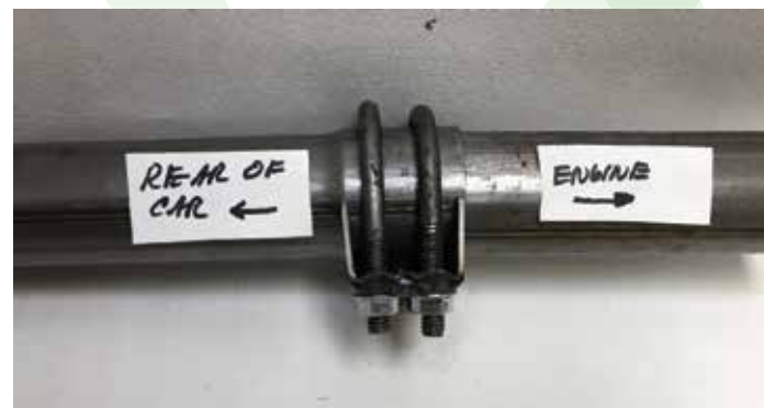
Double clamp on female pipe Two different ways to install the special double clamp.
