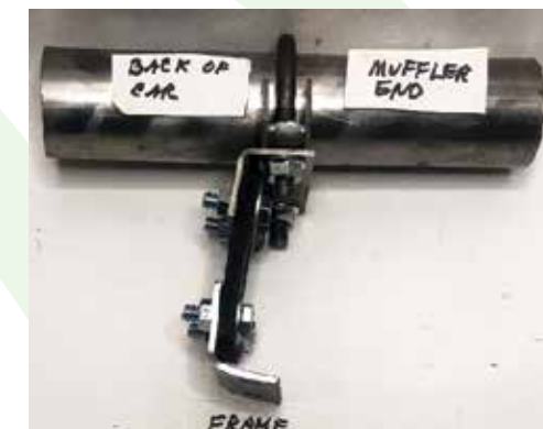
This picture shows the proper placement as they are assembled. All parts of driver side of car.
