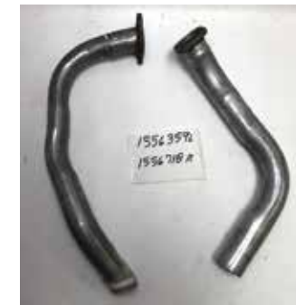
1st pipes (Head Pipes) Studebaker
