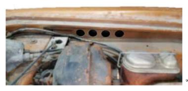
under the hood temperature. It didn't seem to work as well as anticipated. If you think about it, as the car is moving down the road, it seems to me that the pressure from under the front fenders would somewhat block the air from exiting these holes. It might help the hot air to escape the engine compartment when the car was not moving.
