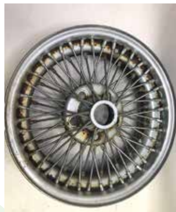
Rusted 6" wire wheel
