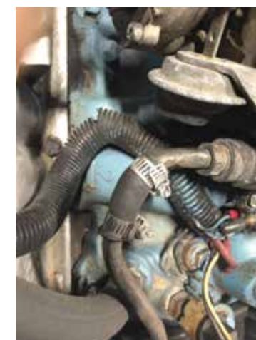
This picture shows the kink was cut out, and a section of rubber hose was installed.
