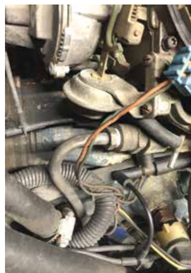
This is a very easy way to tell if you need a new fuel line. First remove the air cleaner, compare the picture to your car, which shows a correct line from the carburetor to the fuel pump.
