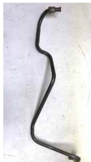
This is a very easy way to tell if you need a new fuel line. First remove the air cleaner, compare the picture to your car, which shows a correct line from the carburetor to the fuel pump.
