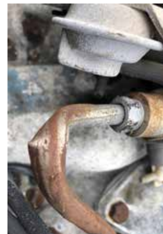
This picture shows a big kink, in the steel line that could leak if the line develops a crack. It obviously restricts the amount of fuel required for proper performance.
