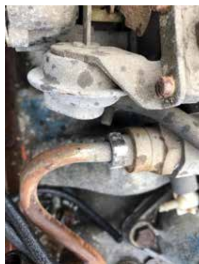
This picture shows the line nut, that the hex is rounded off, which is very common. It makes it difficult to tighten the line nut to the fuel filter cartridge so that it won't leak.
