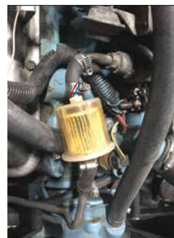
This picture shows the kink was cut out, and an in line fuel filter was installed with two pieces of rubber hoses,
